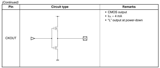
Note: For XIN pin and XOUT pin, refer to "■ OSCILLATION CIRCUIT".
